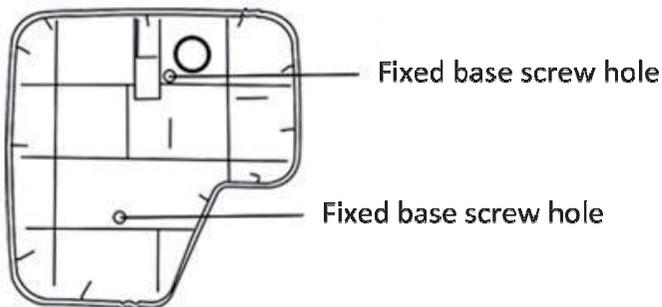
1. Loosen the screws to remove the back plate from the front cover and use it as a template to mark the two holes to be drilled.
